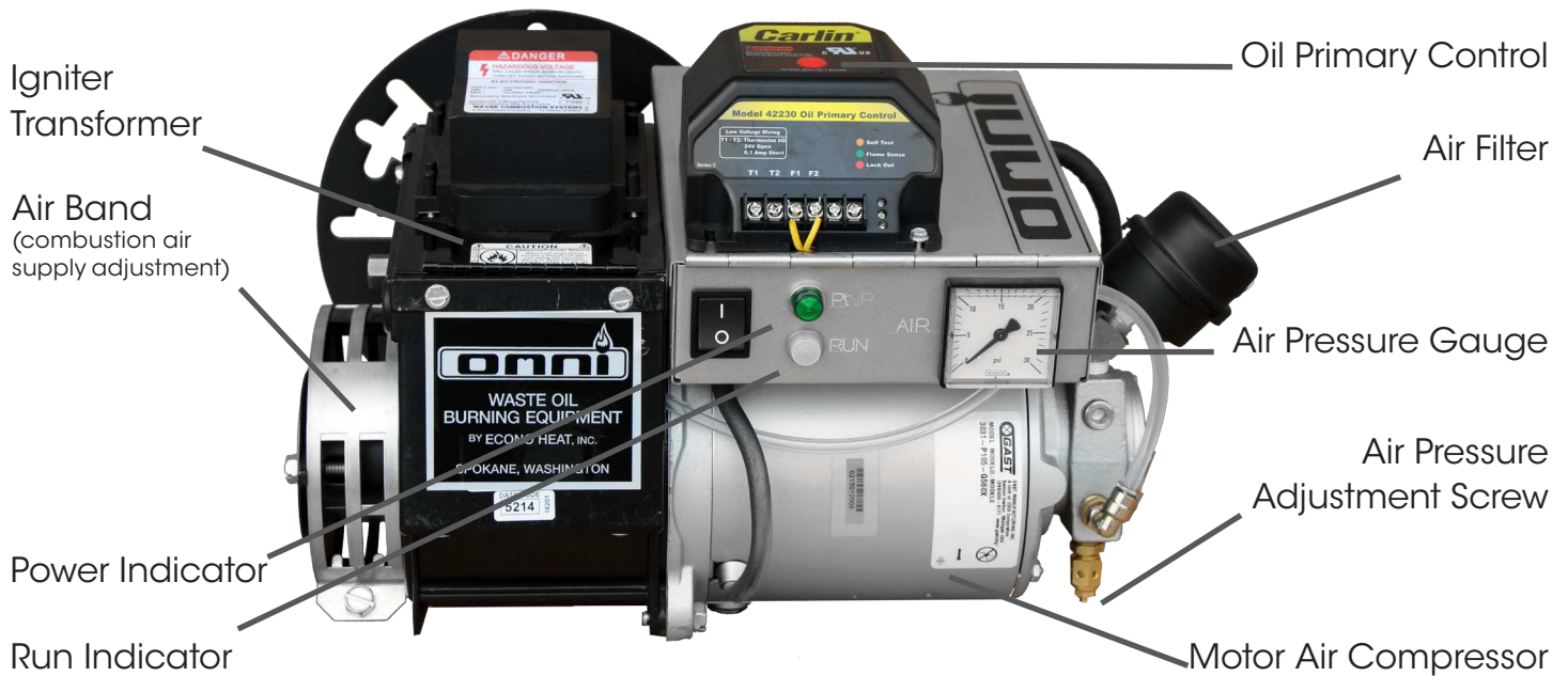
Figure 3 – Oil Burner (Back View Closed)
