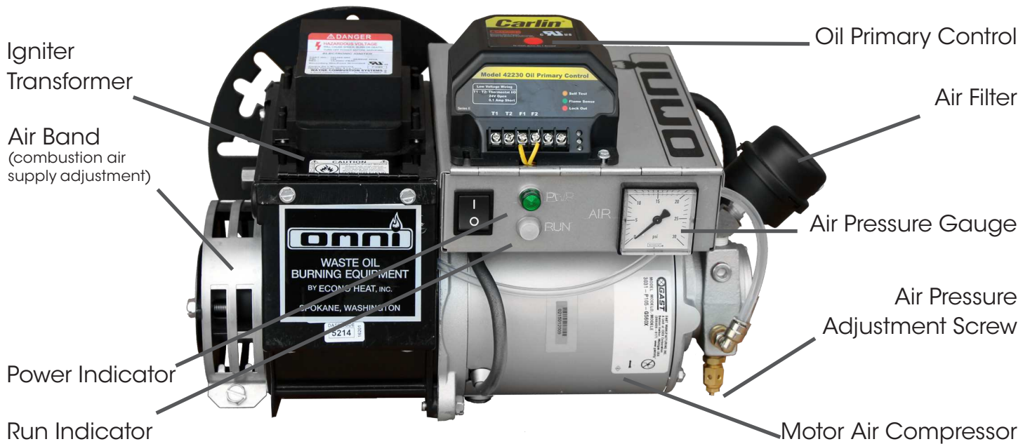
Figure 3 – Oil Burner (Back View Closed)
